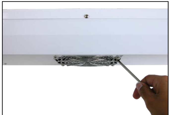
Figure 8. Shorting the ionizer’s two fan grills
