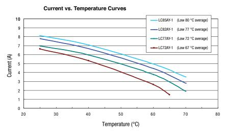
The above curves were derived from placing test samples in an oven at 25 °C, 40 °C, 60 °C and 70 °C, increasing current flow through the sample at a rate of 0.1 A/minute and recording the current value when the sample trips.
