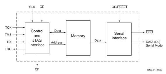
Figure 1: XCFxxS Platform Flash PROM Block Diagram
