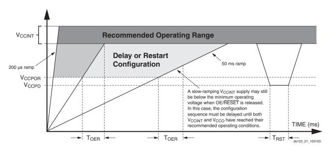
Figure 16: Platform Flash PROM Power-Up Requirements
