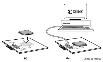
Figure 3: JTAG In-System Programming Operation
