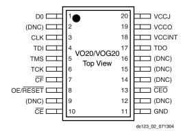
Figure 17: VO20/VOG20 Pinout Diagram (Top View) with Pin Names
