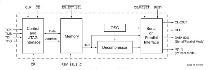
Figure 2: XCFxxP Platform Flash PROM Block Diagram
