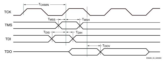
Figure 6: Test Access Port Timing
