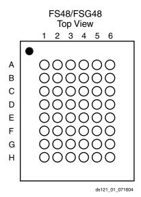
Figure 19: FS48/FSG48 Pinout Diagram (Top View)
