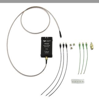
The RP4060 and RP2060 probes are designed specifically to probe low-impedance DC power/voltage rails. Low attenuation means a low-noise view of small signal variations at high frequency, while the probe's built-in offset of up to ±60V enables compensation for the rail's DC voltage. The probe's high DC input impedance eliminates loading of the low-impedance DC rail.
