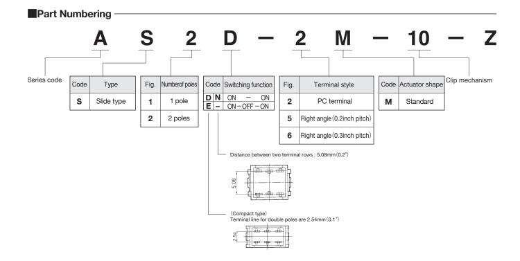
Please refer to P.497 for soldering specifications, flux cleaning, and packaging specifications. Please refer to P.500 for PC hole layouts.
