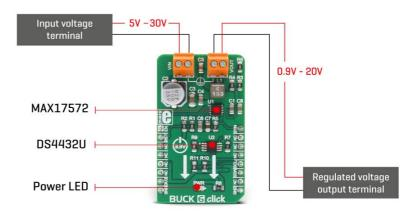
The MAX17572 features a robust overload and short circuit protection. When the internally set current limit of 1.7A is exceeded, the high side MOSFET is turned off and the hiccup mode is triggered. This mode suspends the operation for 32,768 duty cycles after which the soft start sequence is reattempted. If the faulty condition is still present and the feedback voltage remains under 0.58V, the switching frequency will be halved to avoid overheating during the restart sequence.
