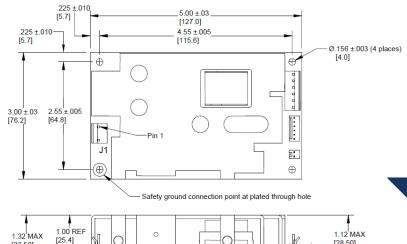
Note: Recommended standoff size is .375" high and all mounting hardware should be less than .28" in diameter. A standoff less than .375" high is acceptable when a thin insulator, 0.4mm thick (polyester, fish paper or equivalent UL rated 94V-2 minimum) is placed between the XR160 and the mounting chassis (refer to applicable UL standard for clearance requirements).
