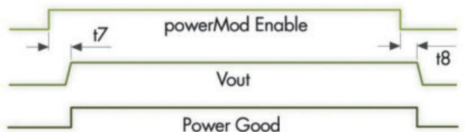
Output powerMod Signals
