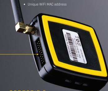
The CODEGRIP device is equipped with the target MCU connector, which contains JTAG/SWD and power supply pins. This connector is used to interface the CODEGRIP device with the target MCU, allowing it to perform programming and debugging operations, to provide the power supply for the target MCU, and to be used as the power input when the CODEGRIP device is powered from the connected development board.
