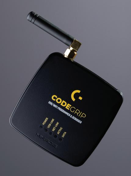
CODEGRIP is a unified solution, designed to perform programming and debugging tasks on a range of different microcontroller devices (MCUs) based on the ARM® Cortex®-M architecture. By bridging differences between various MCUs, it allows a huge number of MCUs from several different MCU vendors to be programmed and debugged. Although the number of supported MCUs is absolutely huge, more MCUs might be added in the future, along with some new functionalities.
