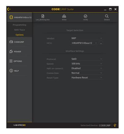
The *Options Menu item* displays a set of options, which are used to select and configure the target MCU.
