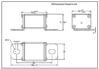
Note: Recommend tightening torque is 12+/-1.0Nm (M8)
