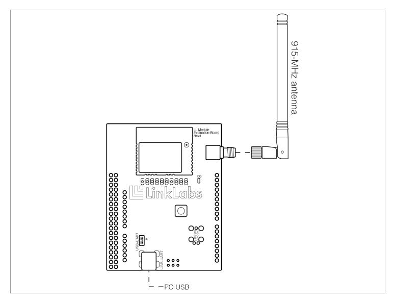
Once connected, a red LED on the evaluation board lights up. This LED lights up anytime the Symphony Link Module has set one or more <u>interrupt request flags</u>. (In this case, the LED indicates a RESET event has occurred because you just supplied power to the board.)
